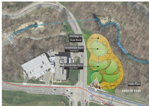
Left: the new green infrastructure installation will receive stormwater from the area inside the box. Above: stormwater will be held in planted basins before discharging into Doan Brook. Photos courtesy of the Northeast Ohio Regional Sewer District
